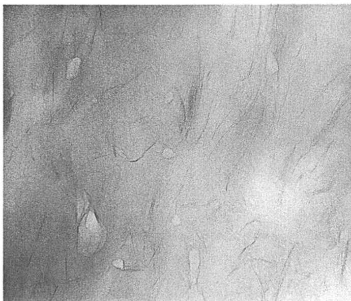
Figure 8. TEM image of PET/5 % DMHdl-MMT nanocomposite
